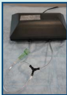
300-gallon aquarium air pump and standard 3/16" aquarium airline tubing
